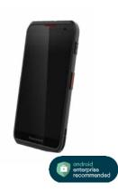
Android 11, 5.5-inch Corning Gorilla Glass touchscreen, 4500mAh battery, 3/32GB, 4/64GB, 6/128GB optional memory, Qualcomm Snapdragon octa-core 2.0GHz processor, Wi-Fi 5, Bluetooth 5.1, 4G LTE connectivity, one nano SIM plus one eSIM, IP67.
